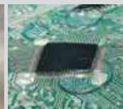
A resin-potted circuit board
